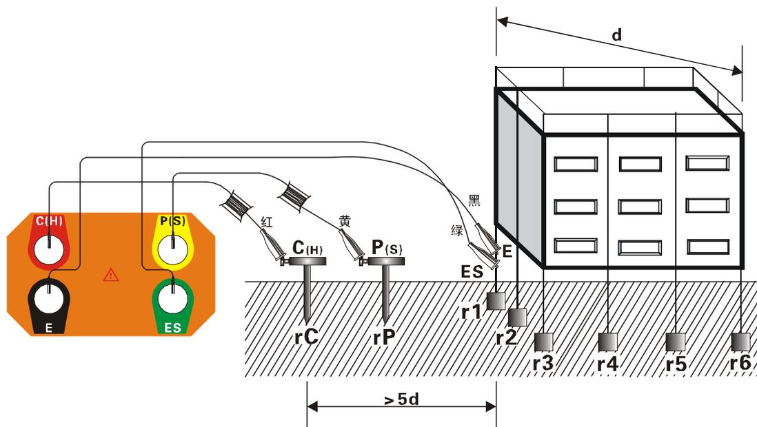
$$R = r_1 \parallel r_2 \parallel r_3 \parallel r_4 \parallel r_5 \parallel r_6 \parallel \dots \parallel r_n \text{ (} r_1 \dots r_n \text{ 都是独立接地点)}$$
